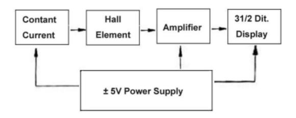
When Hall element H is placed in the magnetic induction field with intensity B and connect a constant current I through end 1 and 3,then a voltage VH would be occurred between end 2 and 4, after amplified by the arithmetic amplifier, it output to the display and the relevant readings of magnetic field intensity will be displayed on the LCD.
